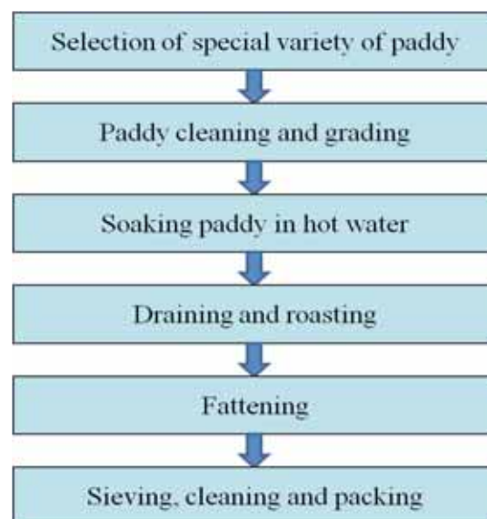
Figure 1. Production process of Chiura in the mills
