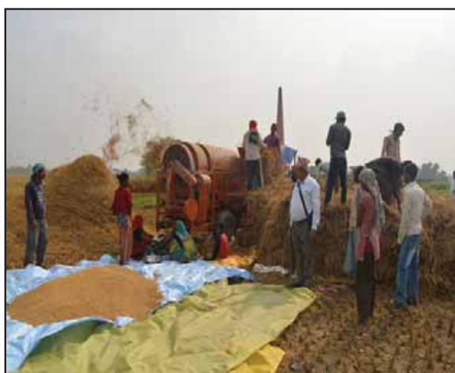
Use of thresher for threshing (Source: BR Sapkota, DoA)
