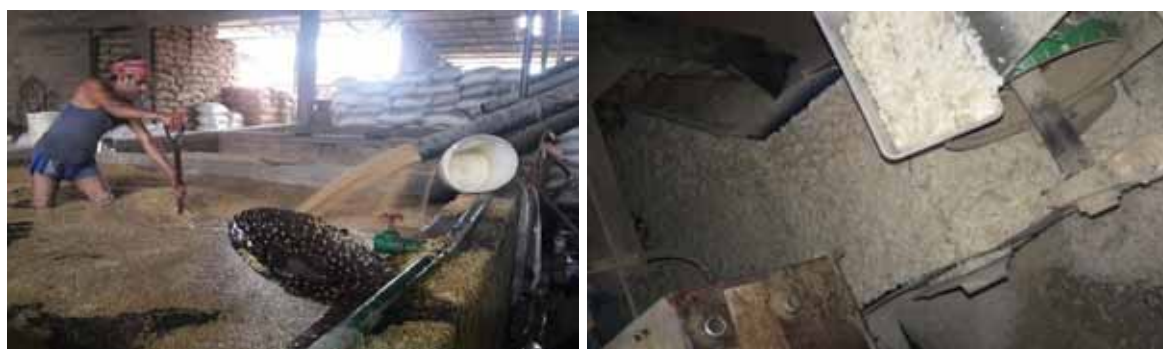
Figure 2. Paddy soaking in water to prepare beaten rice beaten rice after processing
