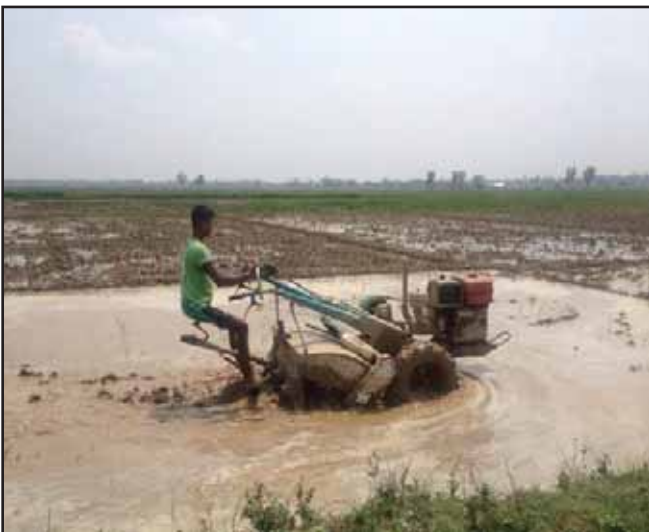
Power tiller use in land preparation (Source: FB of Krishna Sharma)
